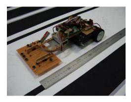
Figure 8. Manufactured line-following robot M3
